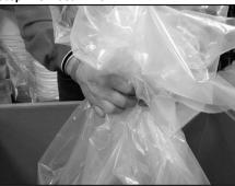
When box is filled, ensure no waste protrudes from box. Gather liner and twist. Secure with provided poly liner tie.
