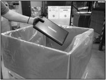
Wearing the proper safety gear, carefully place intact electronics into lined box. DO NOT PLACE BROKEN ELECTRONICS INTO THIS BOX. If the intact electronic device contains a battery, please package to ensure that the device cannot be activated during shipment.
