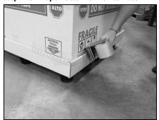
Using 3" pressure sensitive tape, securely tape the bottom of the box to the base. Ensure to tape completely around the container.
