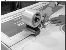
Fold top flaps of box in order marked and tape to seal. Make sure to tape along the length and width.
