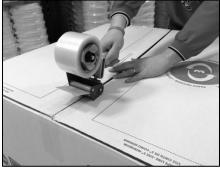
Fold flaps on bottom of box in order marked and tape to seal. Make sure to tape along the length and width.
